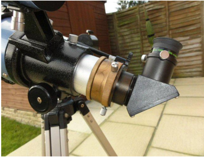
The focusing unit showing adjusting Knobs
