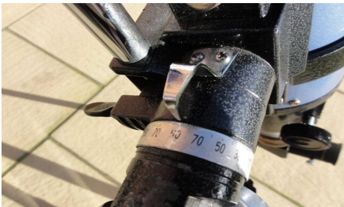
The Declination (Dec) Indicator Barrel
