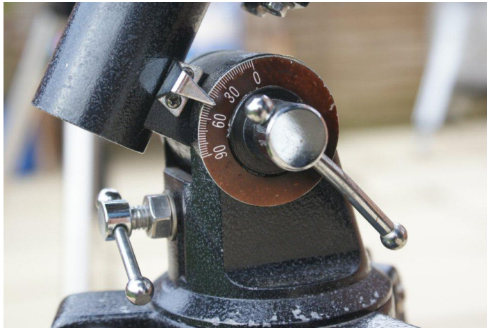
The RA angle adjustment mechanism on an EQ1 Mount
